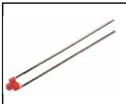
subminiature LED Dome is 1.8mm diameter
