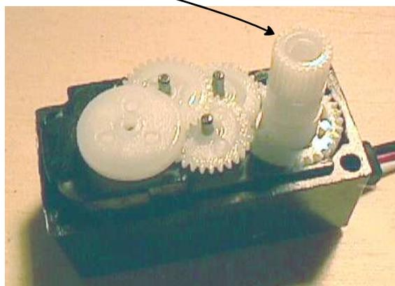
Disconnecting the potentiometer from the drive train means that the servo can never achieve the 'null point' balance it normally looks for and so it will keep rotating. You MUST remember to cut off the rotation stop on top of the final drive gear !!
